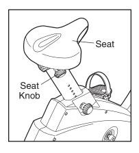
loosen it. Slide the seat forward or backward to the desired position, and then firmly tighten the seat knob.
